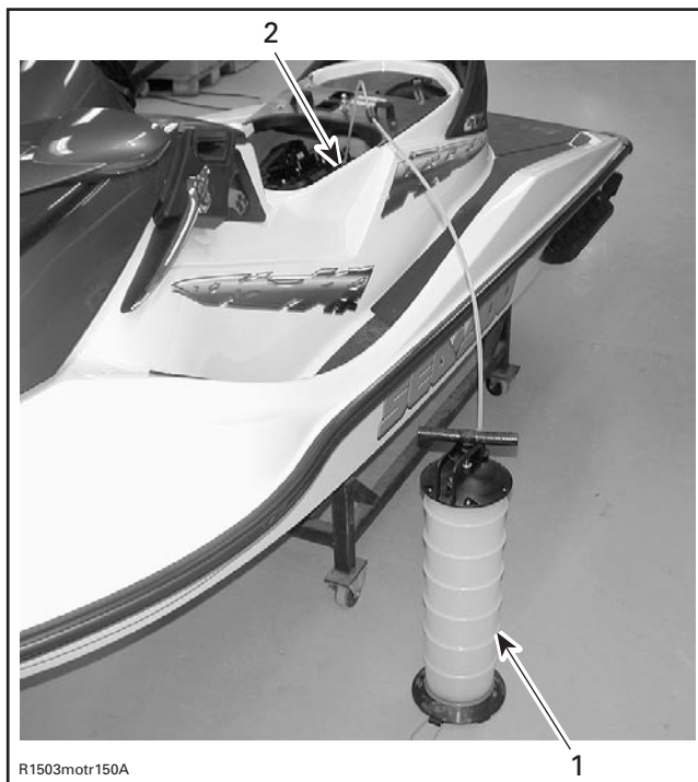
1. Suction pump 2. Siphon tube in dipstick hole
