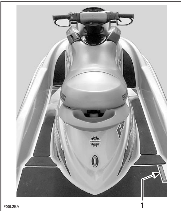
TYPICAL 1. Hull Identification Number (H.I.N.)
