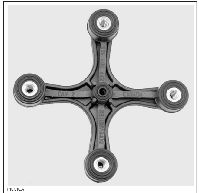
GASKET INSTALLED ON SUPPORT PLATE
