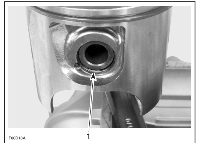
1. Circlip opening at 6 o'clock (at bottom)
