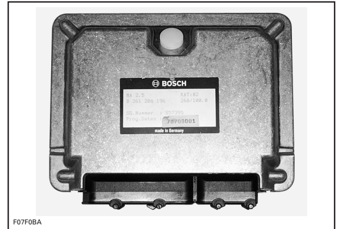
ELECTRONIC CONTROL UNIT (ECU)
