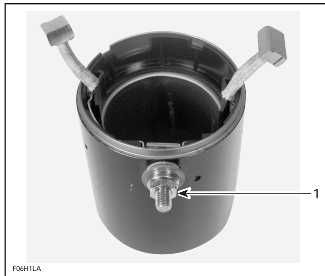
1. Loosen nut and remove washers
