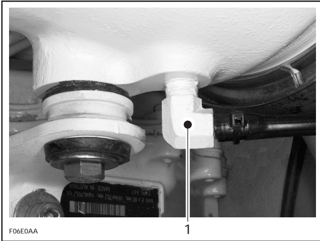
1. Water injection hose
