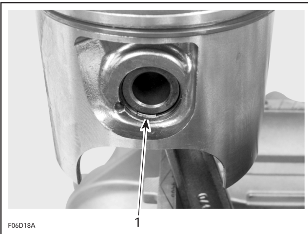
F06D18A 1. Circlip opening at 6 o'clock (at bottom)
