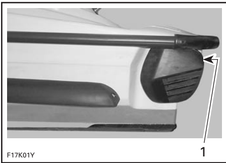
1. Side vane in upper position
